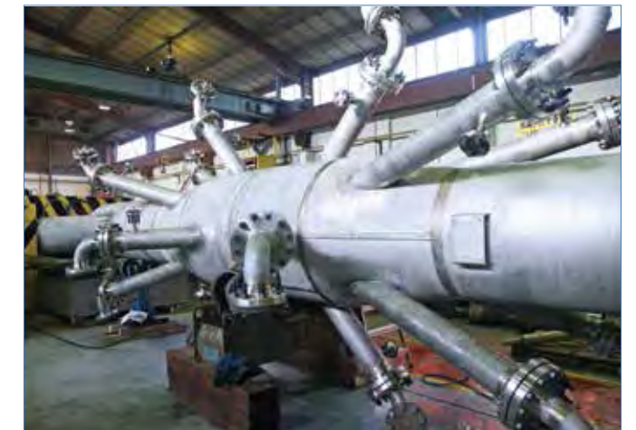
Quench fitting in stainless steel 321H
