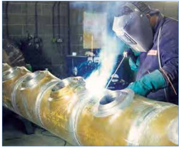
The world's first bimetallic wellhead manifold in X65 clad with alloy 825
